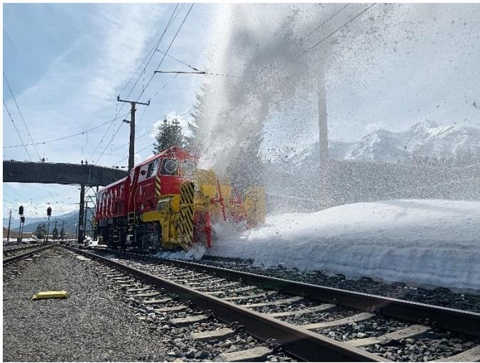
*Thanks to MAN power, the Schmidt Beilhack HB1100S clears up to 10,000 tons of snow per hour.*
