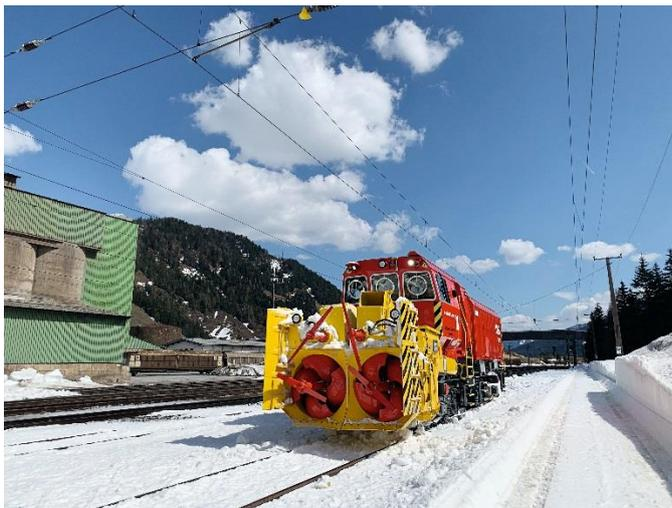
*Schmidt Beilhack HB1100S on the test track in Hochfilzen. One of the two 793 kW MAN engines is required just to power the blower, which can be clearly seen in the foreground.*
