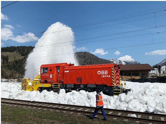
*Schmidt Beilhack HB1100S heavy snow blower during start-up in Hochfilzen, Austria. The two MAN twelve-cylinder engines are installed in the rear of the machine.*
