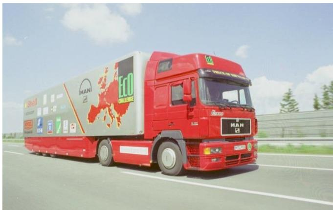
In 1995, even this record was broken. A consumption benchmark for 40-tonne articulated trucks previously believed impossible was achieved by the Eco-Challenge Tour 1995. Due to its aerodynamic panelling and trained drivers, an MAN F2000 tractor-trailer travelled from Edinburgh to Bari in southern Italy, while utilising merely 25.2 litres of diesel per 100 kilometres – a world efficiency record at the time!
