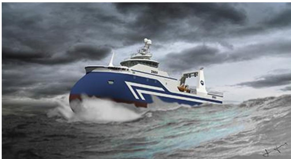
*Graphic representations of the Nautic wetfish trawler design for HB Grandi. Each vessel will be powered by an MAN six-cylinder L27/38 unit, accompanied by a four-bladed, 3.8-metre, ducted MAN Alpha VBS 860 propeller (Both images courtesy of HB Grandi/Nautic)*
